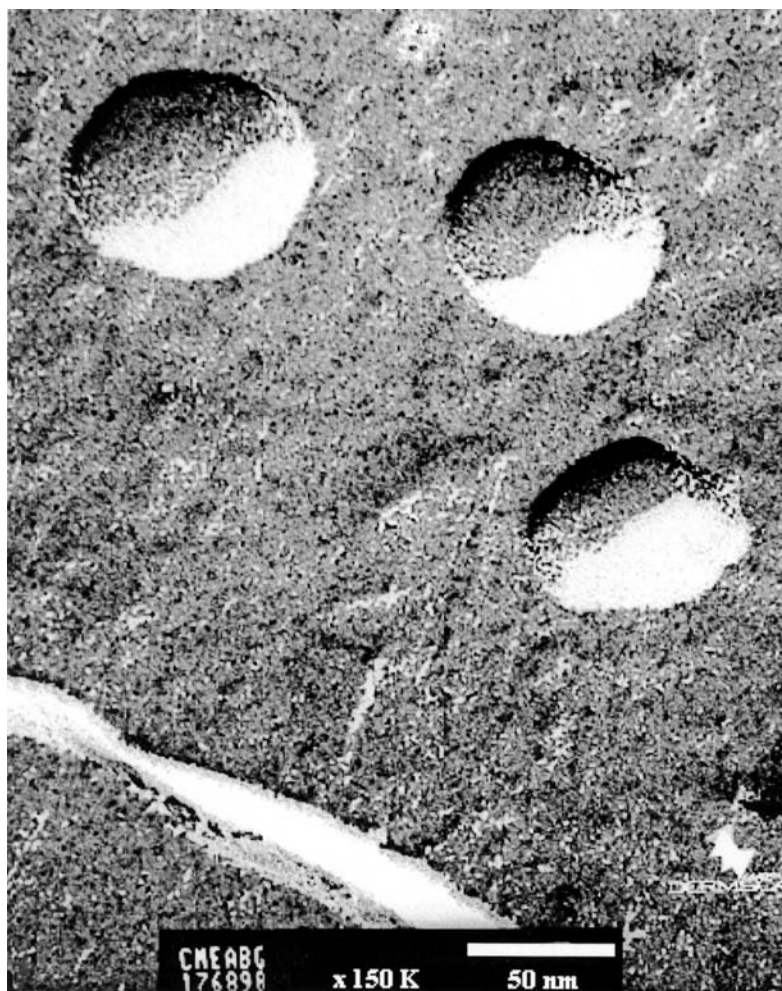
Fig. 4. Cryofracture Transmission Electron Microscopy ( \times 150,000 ) of PSC in water.
